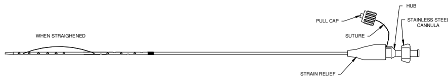
Figure 2 – Catheter Assembled for Insertion (shown with stainless steel cannula)
