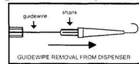
**Caution:** DO NOT grasp and pull the guidewire prior to releasing the Captive® J-Straightener. Damage to the guidewire may occur if it is pulled against the restraint of the Captive® J-Straightener.
