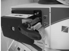
**Tubing Set and Reusable Occlusion Bed installed in the IntelliFlow Pump**
